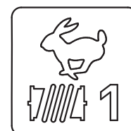
Main winch high-speed hoist down (on MFD)
